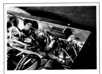
Close-up of underside showing the rectifier sockets and the new 25-watt resistor mounted on the rear apron.
